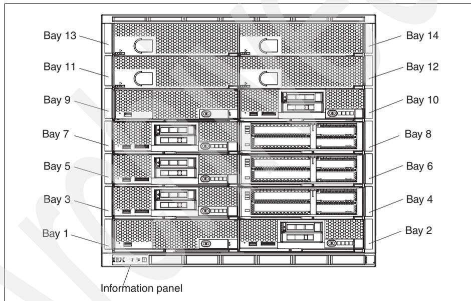
Figure 3-2 Enterprise Chassis - front view
