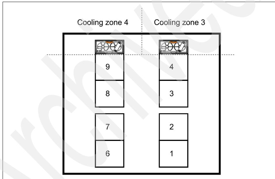
Figure 3-8 Enterprise Chassis switch module and Chassis Management Module cooling zones 3 and 4
