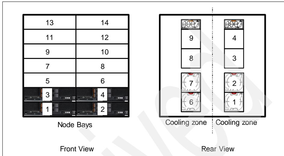
Figure 5-13 Four 80 mm fan modules support a maximum of four half-wide nodes installed
