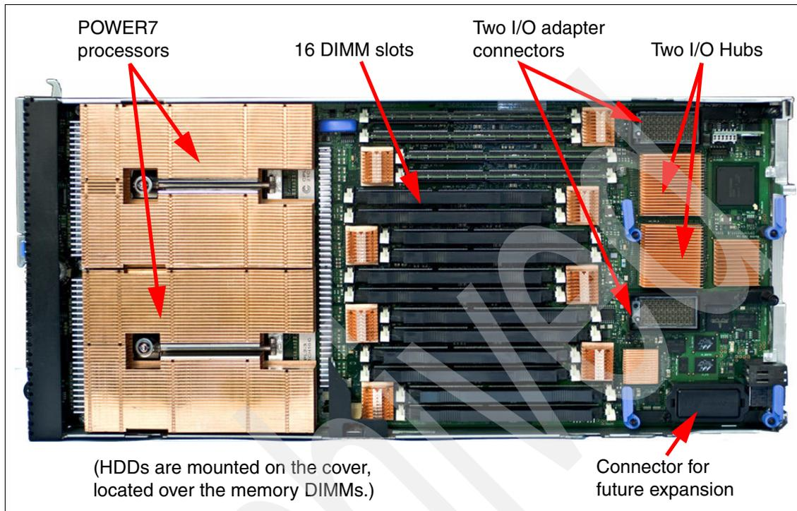
Figure 4-2 System board layout of the IBM Flex System p260 Compute Node
