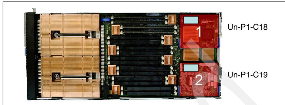
Figure 7-16 p260 adapter location codes
