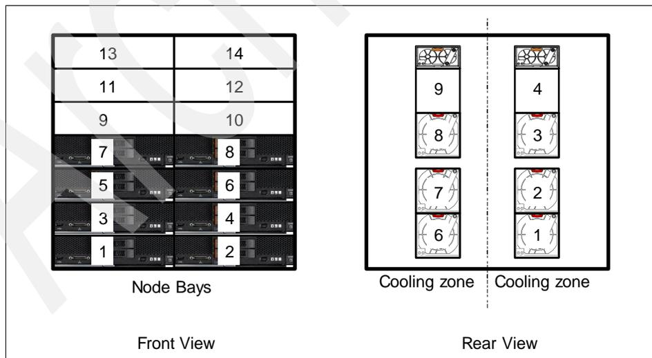
Figure 5-14 Six 80 mm fan modules support a maximum of eight half-wide nodes
