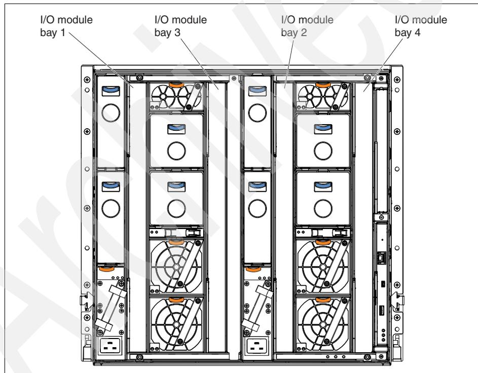
Figure 3-3 Enterprise Chassis I/O module locations
