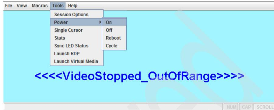
Figure 6-46 Powering on the FSM from the remote console session
