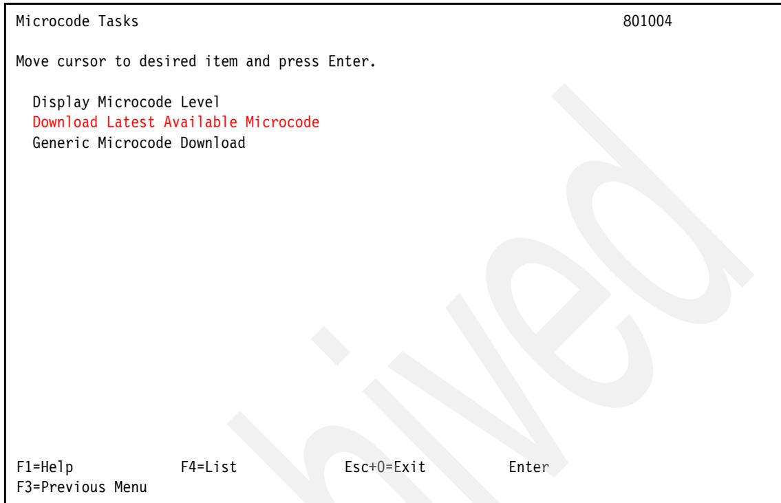
Figure 8-5 Download (install) the latest available microcode
