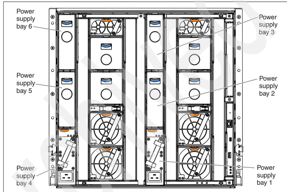
Figure 5-9 Power supply location
