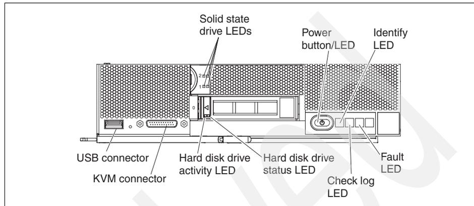
Figure 6-40 FSM front panel - controls and LEDs
