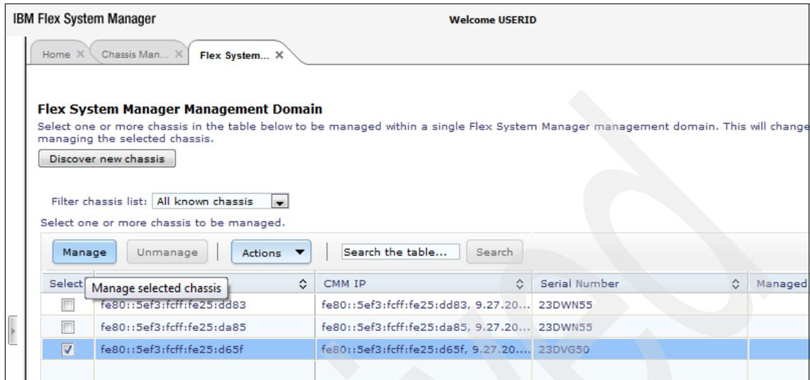
Figure 6-78 FSM chassis selection for management
