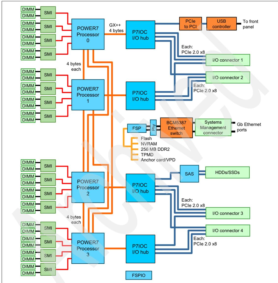
Figure 4-10 IBM Flex System p460 Compute Node block diagram
