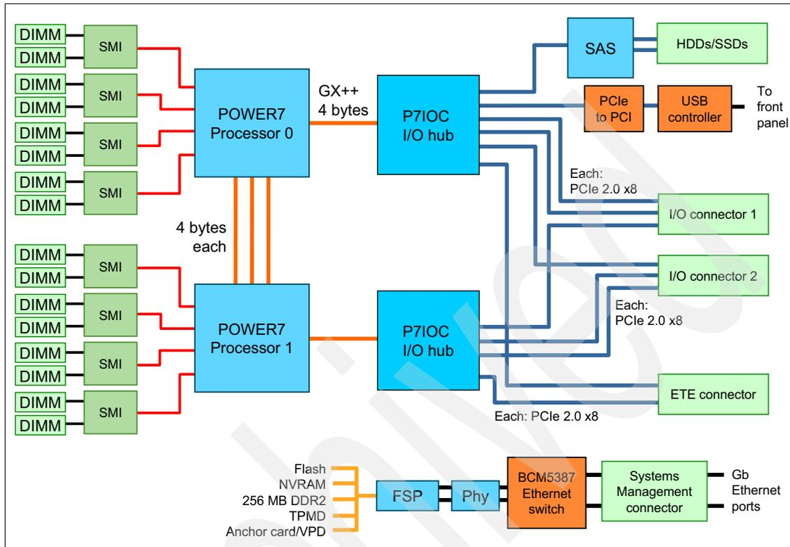
Figure 4-9 IBM Flex System p260 Compute Node block diagram
