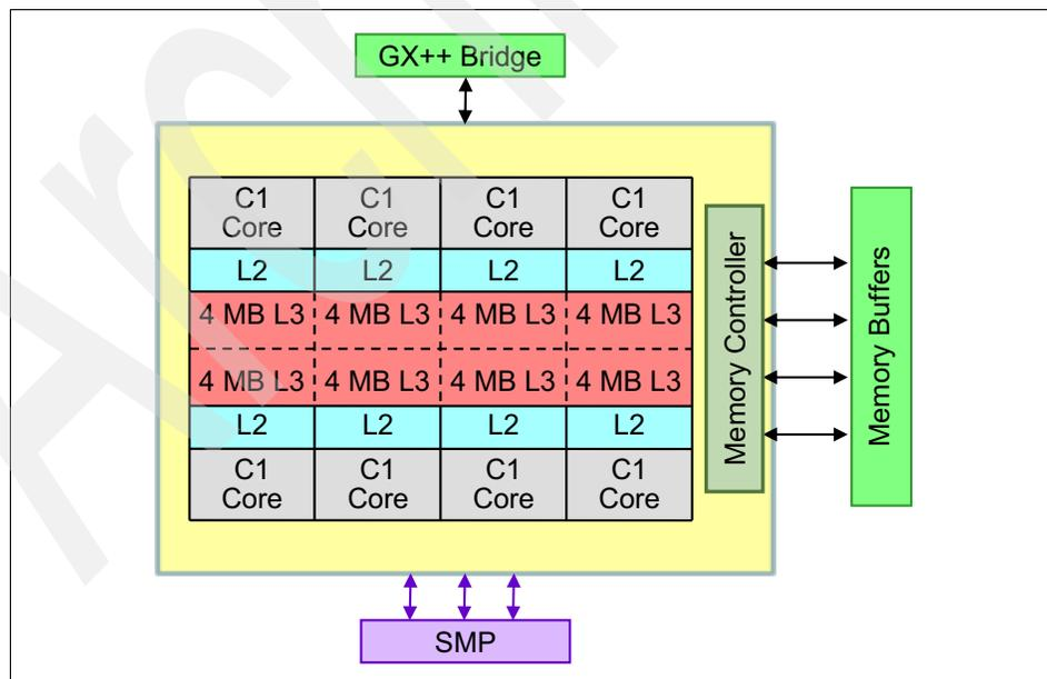
Figure 4-12 POWER7 processor architecture
