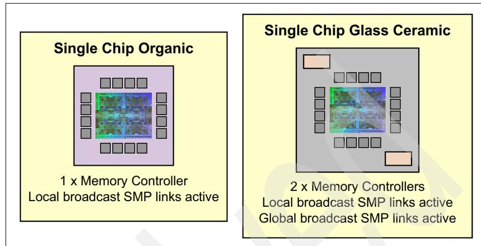
Figure 4-15 Outline of the POWER7 processor physical packaging
