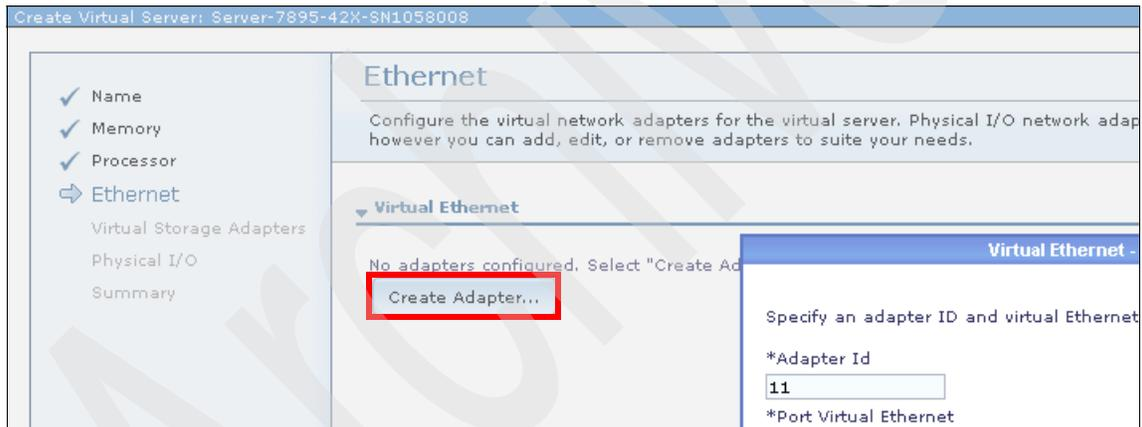
Figure 7-10 Create the bridging virtual Ethernet adapter in the VIOS
