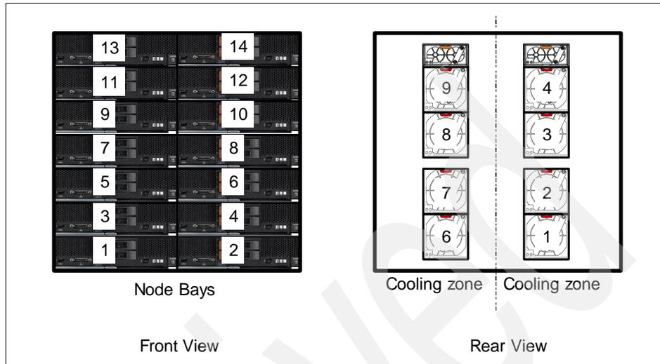
Figure 5-15 Eight 80 mm fan modules support from 7 to 14 nodes
