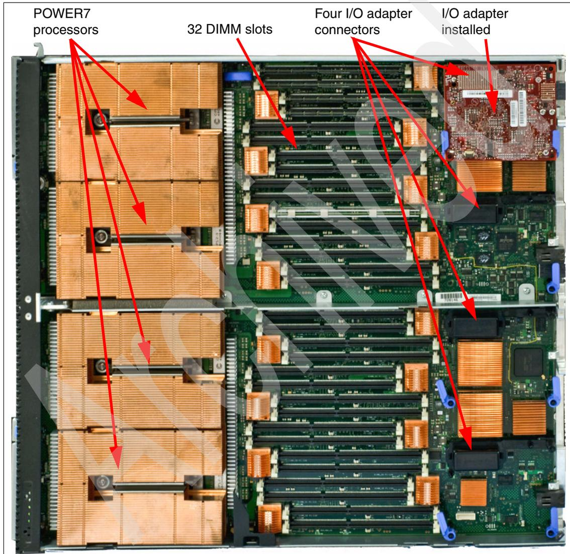
Figure 4-3 System board layout of the IBM Flex System p460 Compute Node
