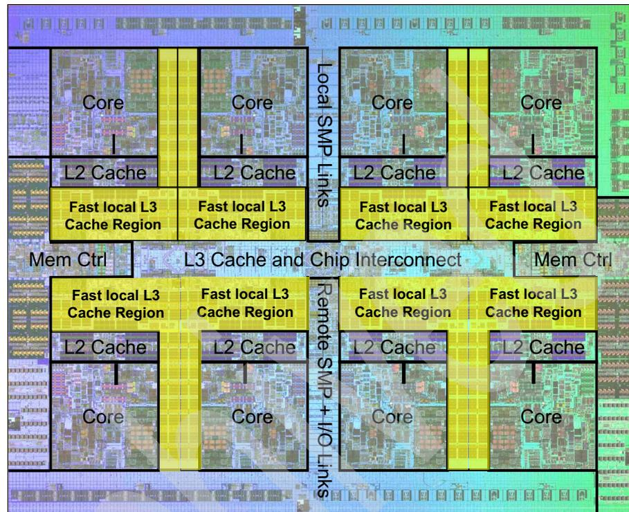
Figure 4-16 FLR-L3 cache regions on the POWER7 processor
