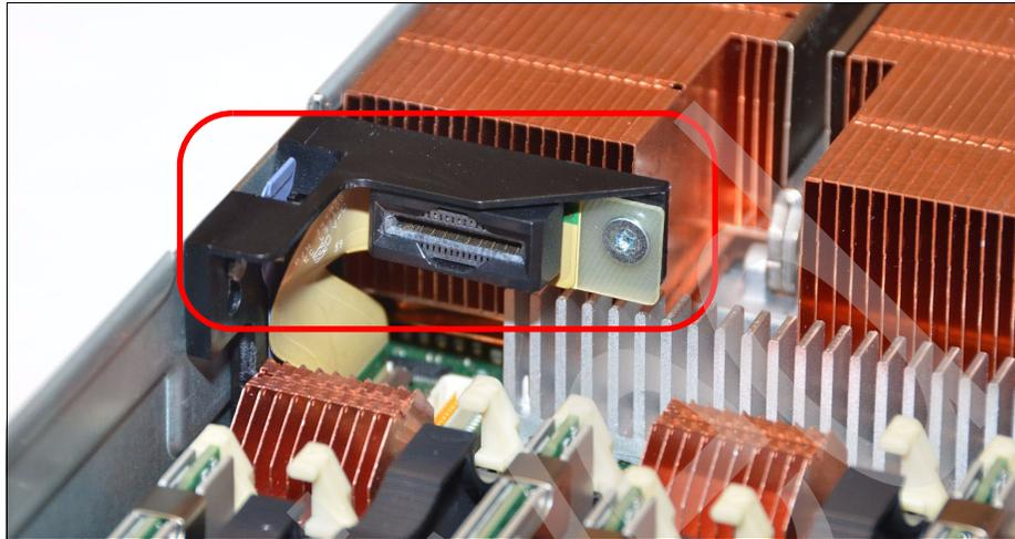
Figure 4-22 Connection for drive interposer card mounted to the system cover (connected to the system board through a flex cable)
