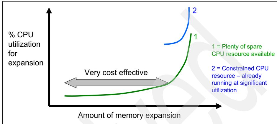
Figure 4-18 Processor usage versus memory expansion effectiveness
